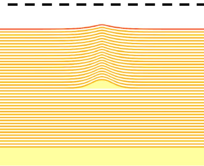
Mask Blank with buried defect
