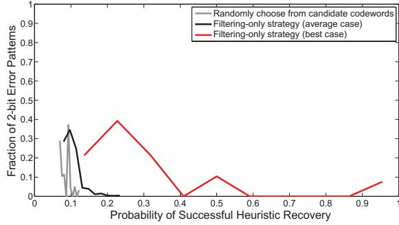
Fig. 6. Baseline histogram of successful rates for heuristic recovery over all 741 possible 2-bit DUE error locations for MIPS instructions in *bzip2* using a (39,32) SECDED code using the *filtering-only* strategy.
