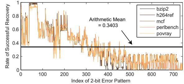
Fig. 8. Rate of successful heuristic recovery for MIPS instruction memory for five benchmarks over all 741 possible 2-bit DUE error locations with a (39,32) SECDED ECC code. Here, we apply the *filtering-and-ranking* strategy, i.e., candidate codewords are first filtered for valid instruction messages before choosing the most-commonly occurring operation as the recovery target.
