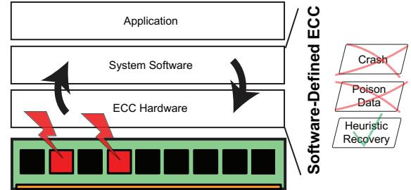
Fig. 1. High-level concept for Software-Defined Error-Correcting Codes (SWD-ECC), which, instead of crashing or poisoning data, heuristically recovers from DUEs that occur in memory words (red lightning bolts) via the collaboration of system software and ECC hardware.
