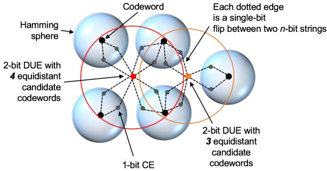
Fig. 2. Conceptual illustration of a two-dimensional partial slice of the  $n$ -dimensional binary space for a general  $(n,k)$  SECDED code. Each point represents an  $n$ -bit string, all of which are either codewords, CEs, or DUEs. Not all DUEs (red and orange points) have the same number of equidistant candidate codewords, as shown by their 2-bit radii (red and orange circles).
