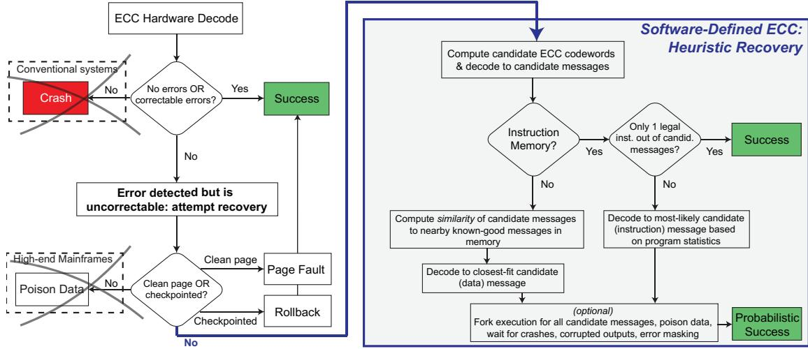
Fig. 3. Proposed system-level flow for Software-Defined ECC.
