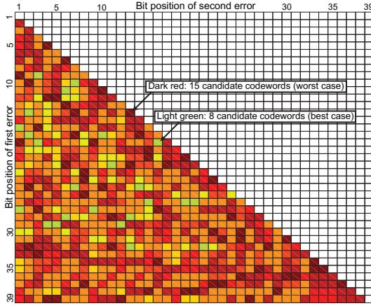
Fig. 4. This heatmap depicts the number of candidate codewords as a function of the two error bit locations in a DUE using our (39,32) SECDED ECC code. Hotter colors indicate more candidates, which range from 8 to 15. There are exactly 741 possible 2-bit error patterns.
