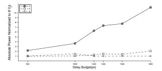
Fig. 16. Optimal powers for varying delay budgets and different  $V_t$  granularities. The powers are normalized to the corresponding results for eight  $V_t$  variants.
