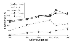
Fig. 14. Suboptimalities for EP-LD model under different delay constraints, using  $V_t$  variants only.
