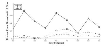
Fig. 13. Optimal power vs. delay budget for different gate size granularities. Power values are normalized to corresponding optimal results for eight gate sizes.
