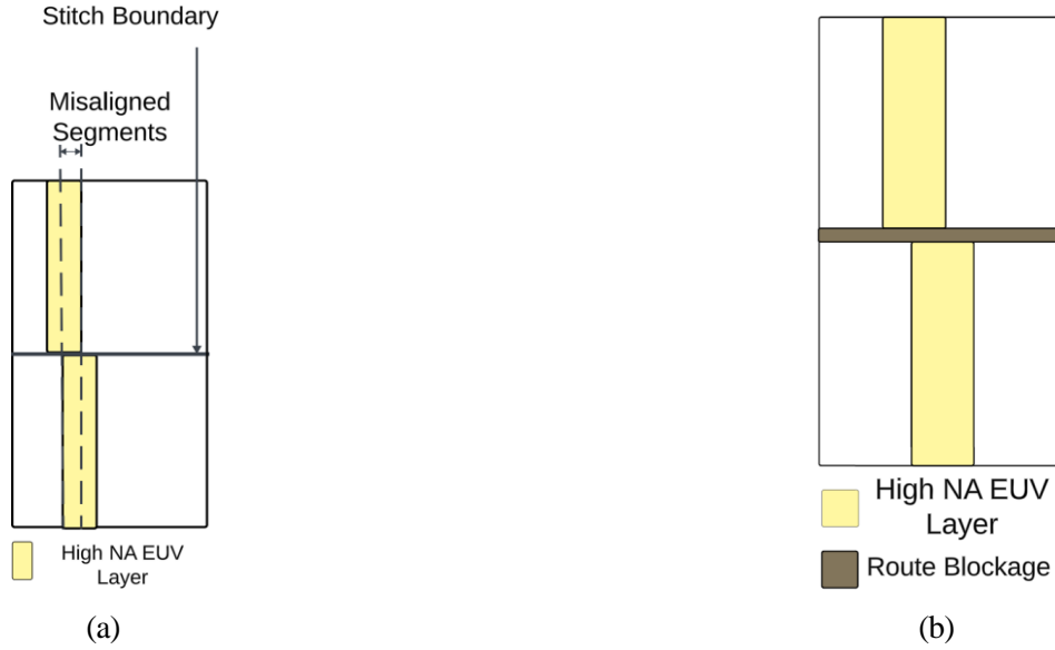
Fig 2: a) Yield Loss Due to Overlay Error b) Proposed Solution - Route Blockage in the Stitch Region
