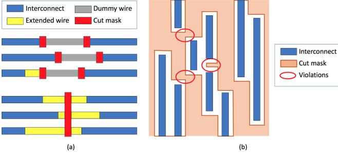
Fig. 9. (a) End cut illustration and optimizations. (b) Block cut illustration and optimizations.
