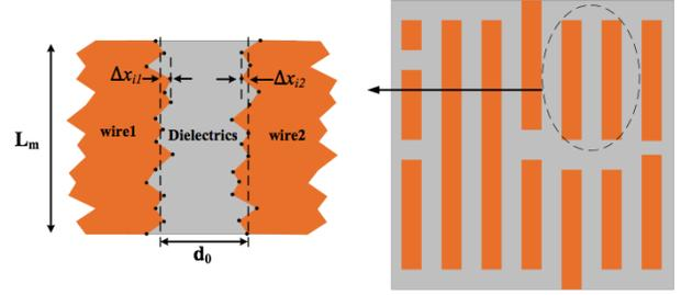
Fig. 3. An illustration of the LER model in this study.
