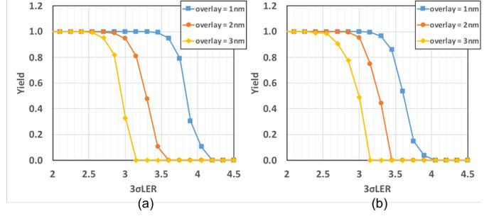
Fig. 11. Yield of (a) AES and (b) CORTEXM0DS MINT1 versus  $3\sigma_{LER}$  for varying overlay mismatch
