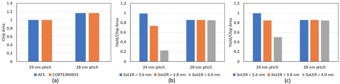
Fig. 16. (a) The estimated chip area when using different wire pitches. (b) Yield/chip area for AES. (c) Yield/chip area for CORTEXM0DS.
