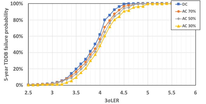
Fig. 12. 5-TDDB failure probability for 24 nm AES MINT1.
