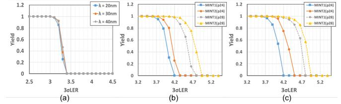
Fig. 6. (a) Yield of 24 nm pitch of 1D wires. (b) Yield of 24 nm pitch of AES. (c) Yield of 24 nm pitch for CORTEXM0DS.
