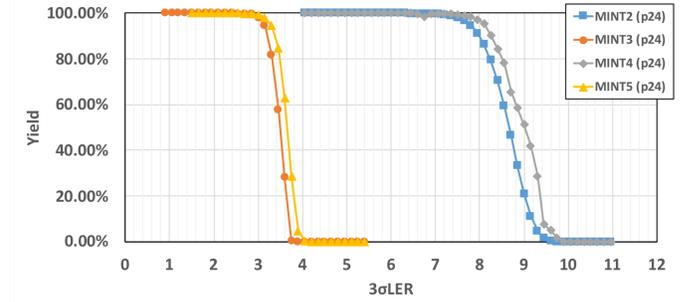
Fig. 10. Yield versus  $3\sigma_{LER}$  for 24 nm and 28 nm pitch trim mask design.
