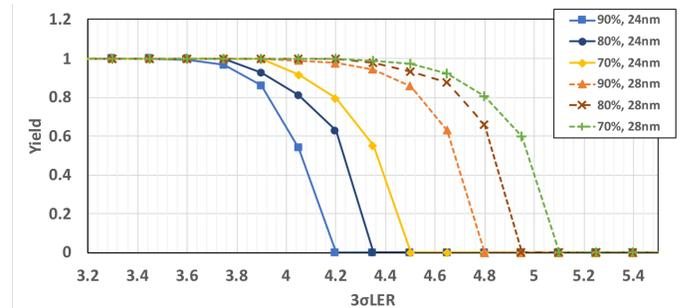
Fig. 8. Yield of CORTEXM0DS MINT1 with differing utilization rates.
