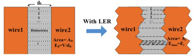
Fig. 4. The model for calculating TDDB failure with segmentation.
