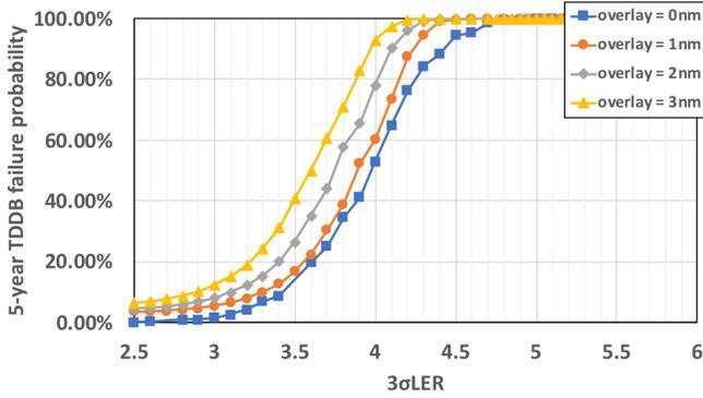
Fig. 13. 5-TDDB failure probability for 24 nm AES MINT1 with overlay.
