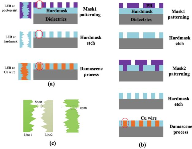
Fig. 2. (a) single patterning by EUV. (b) litho-etch litho-etch patterning by EUV. (c) An illustration of LER induced wire shorts and opens.
