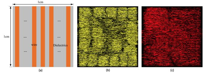
Fig. 5. (a) 1D metal pattern. (b) MINT1 layout for AES. (c) MINT1 layout for CORTEXM0DS.
