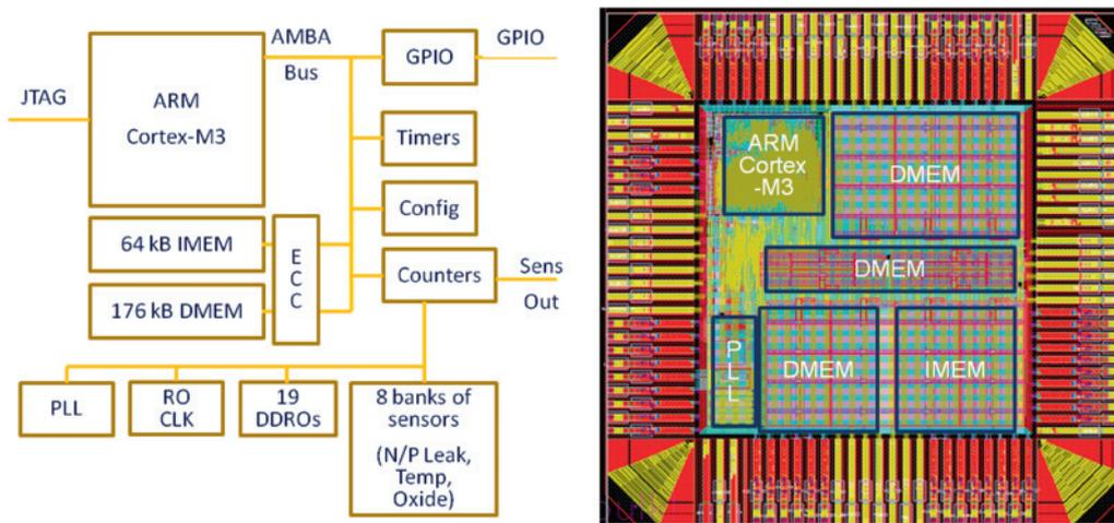
Figure 16: Ferrari testchip block diagram and layout illustration.
