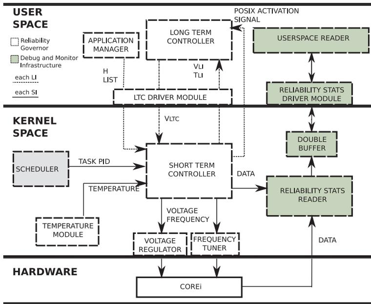
Figure 14: Block diagram for the Linux reliability governor.
