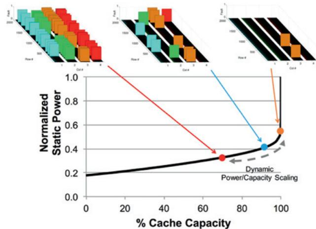
Figure 12: Dynamic Power/Capacity Scaling for SRAM caches.
