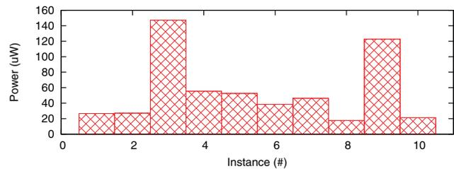
**Figure 1:** Cortex-M3 (Atmel SAM3U) sleep power at room temperature.
