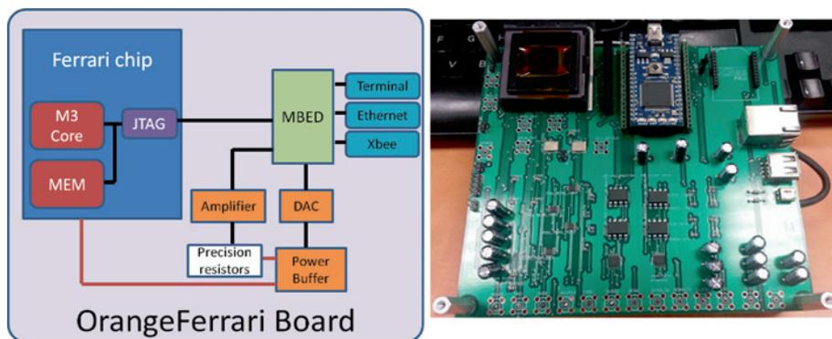
Figure 17: OrangeFerrari testbed block diagram and board photo.
