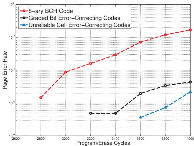
Figure 6: Page error rates in flash with different coding schemes.
