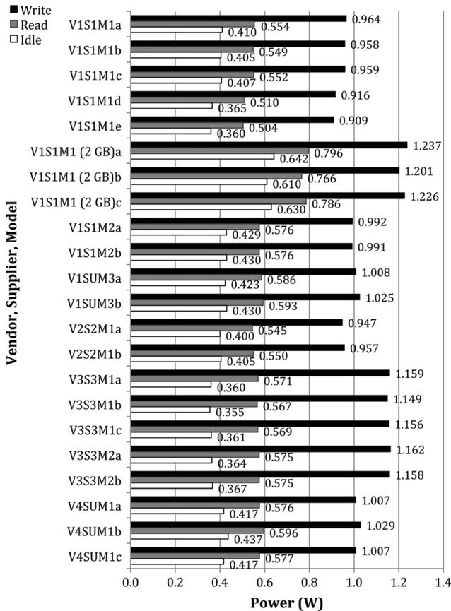
Fig. 3. Write, read, and idle power by DIMM,  $30^{\circ}\text{C}$ .
