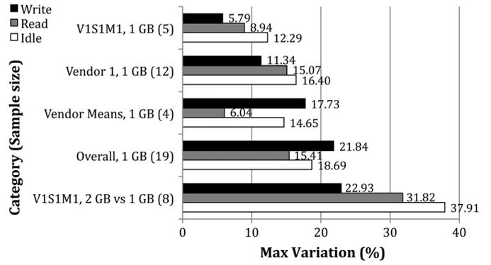
Fig. 4. Maximum variations in write, read, and idle power by DIMM category,  $30^{\circ}\text{C}$ .
