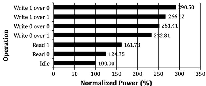
Fig. 1. Data and operation dependence of DIMM power.
