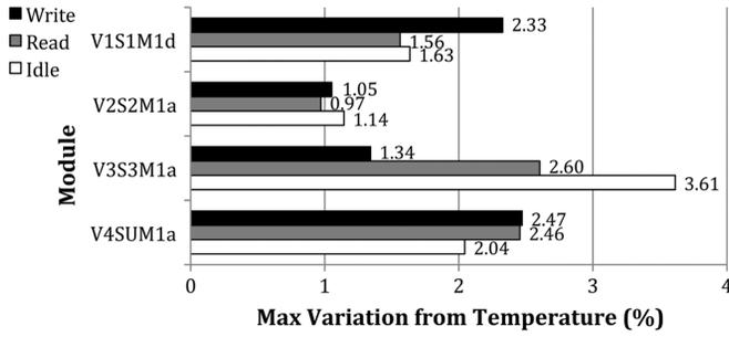
Fig. 2. Relative temperature effects on write, read, and idle DIMM power,  $-50^{\circ}\text{C}$  to  $50^{\circ}\text{C}$  Range.
