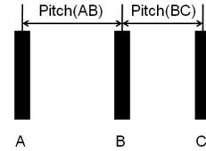
Figure 2. Example illustrating gate-pitch restriction. In case  $Pitch(AB)$  is  $< X_0$  but different than  $X$ , then  $Pitch(BC)$  must be either  $X$  or  $\geq X_0$  and  $Pitch(AC)$  must be  $\geq X_0$ . Similarly, if  $Pitch(BC)$  is unrestricted,  $Pitch(AB)$  is restricted to  $X$  or  $\geq X_0$  and  $Pitch(AC)$  to  $\geq X_0$ .
