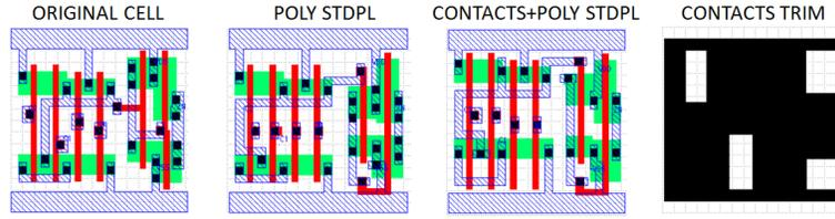
Figure 6. Example of 4-input OAI cell layout migrated for the application of ST-DPL at the poly and CA layers with  $1.8\times$  pitch relaxation.
