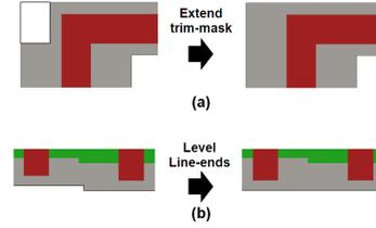
Figure 9. Trim-mask notch-fill by (a) trim-mask extension and (b) poly line-end leveling.
