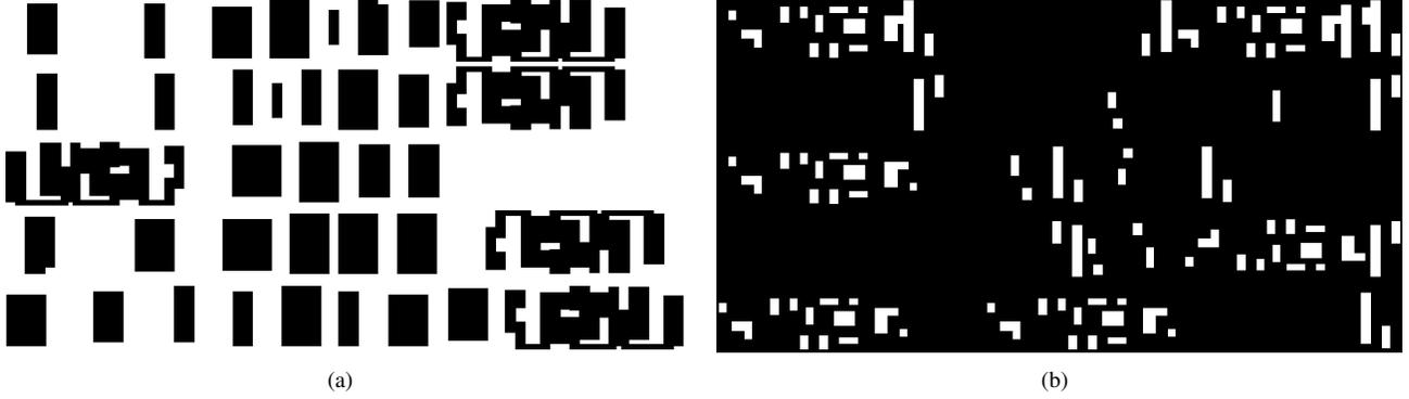
Figure 10. Trim-mask layout snippet for poly-lines (a) and contacts (b). In (a), simple large blocks correspond to cells with unidirectional poly-lines and more complex shapes correspond to flip-flops with bidirectional poly-routing. In (b), both flip-flop and combinational logic regions have simple trim-mask features.
