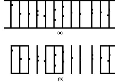
Figure 3. Poly layer ST-DPL critical mask snippet corresponding to a flip-flop cell with two structure-options (a) and (b).
