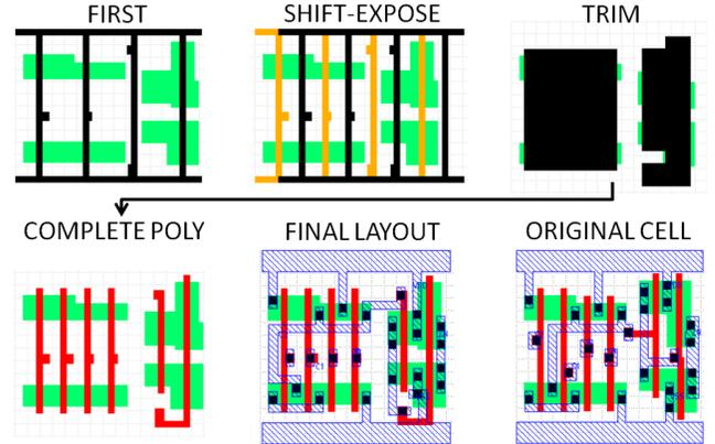
Figure 4. Example of 4-input OAI cell layout migrated for the application of ST-DPL at the poly-line layer.
