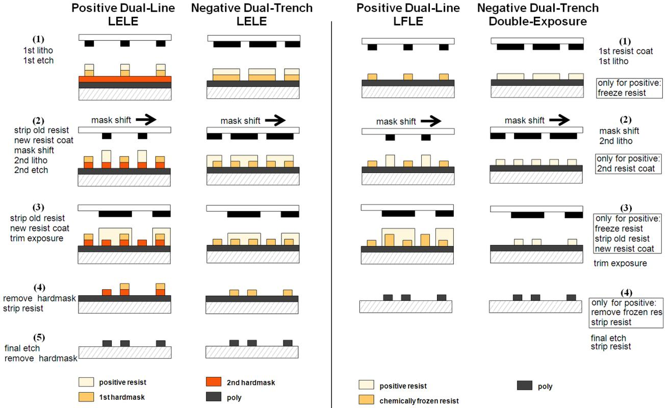
Figure 1. Proposed manufacturing processes for ST-DPL: positive dual-line and negative dual-trench LELE, positive dual-line LLE, a.k.a. litho-freeze-litho-etch (LFLE) process, and negative dual-trench double-exposure processes.
