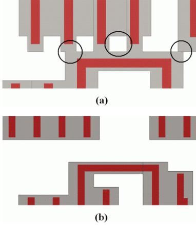
Figure 8. Trim-mask complexity at cell-boundaries before (a) and after (b) enforcing rules (2) and (3).
