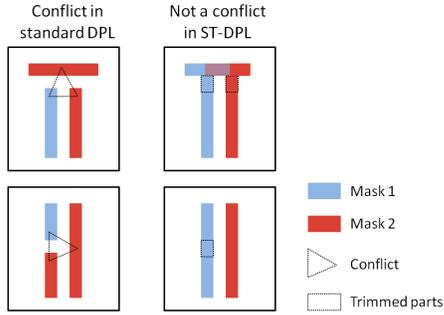
Figure 5. Examples showing how the trim exposure resolves decomposition conflicts.
