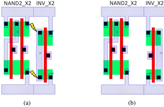
Figure 11. Example of layout decomposition conflicts (marked with the arrows) between features of different cells (a) and our correct-by-construction cell layout that guarantees no conflicts (b).
