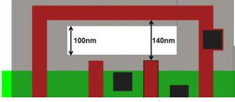
Figure 7. Poly line-tip to poly side spacing rule of 140nm to ensure a minimum hole width of 100nm.
