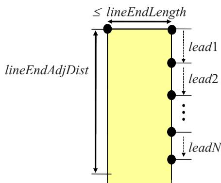
**Fig. 12** OPC parameters for line-end fragmentation.
