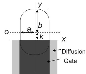
Fig. 3 An example of line-end shape represented by the super-ellipse equation.
