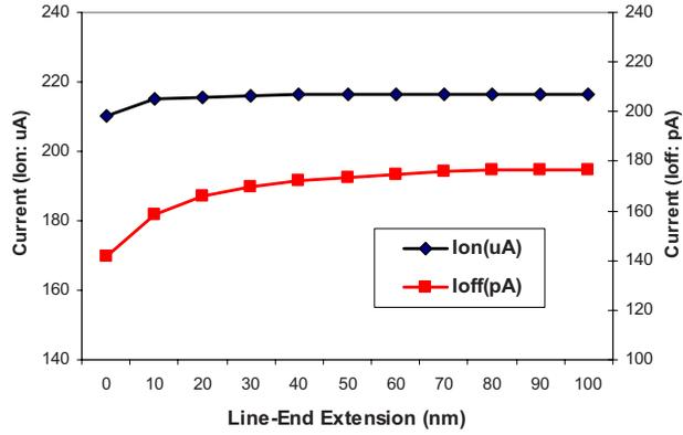
Fig. 1  $I_{on}$  and  $I_{off}$  change due to line-end extension length.
