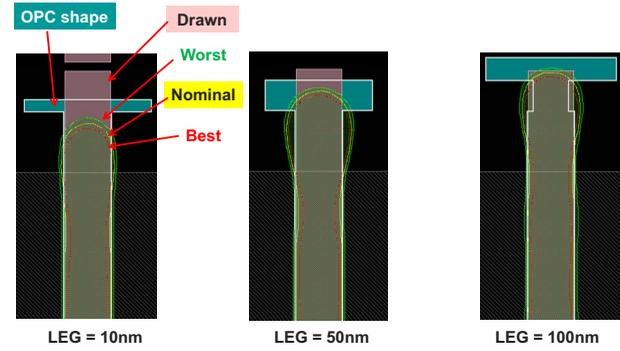
**Fig. 16** Litho contours at best-case (red), nominal-case (yellow), and worst-case (green) process corners, for 10-nm, 50-nm and 100-nm LEG rules. (Color online only.)
