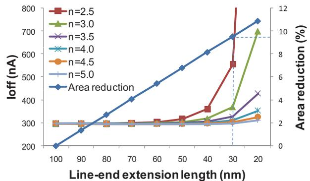
**Fig. 11** Area-leakage trade-off for a logic cell.
