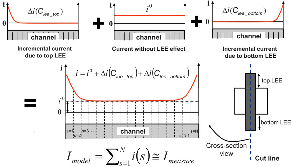
Fig. 6 Nonuniform channel modeling procedure.
