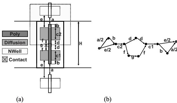
**Fig. 10** Inverter cell layout and height constraint graph. (a) Standard logic layout. (b) Height constraint graph.
