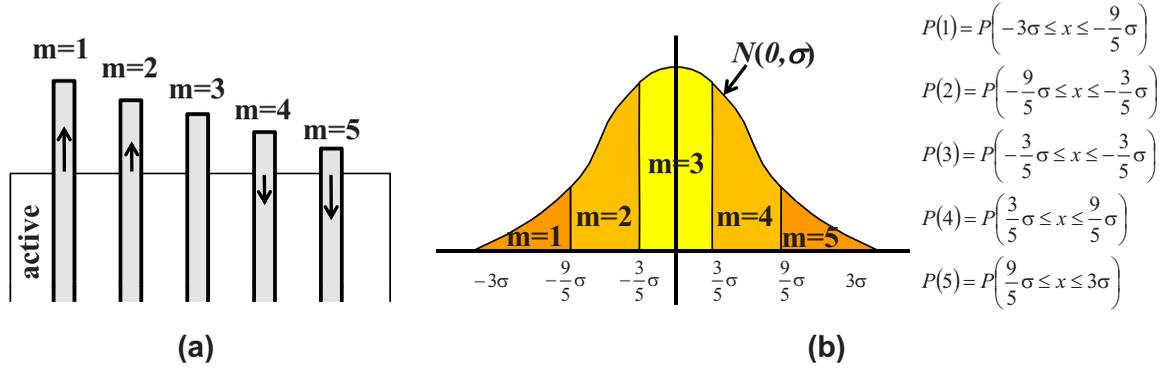
Fig. 7 Overlay error model: (a) five discretized overlay errors, and (b) probability  $P(m)$  calculation for each overlay error  $m$ .
