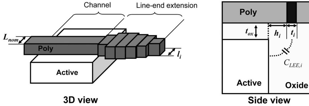
Fig. 4 Modeling line-end capacitance.
