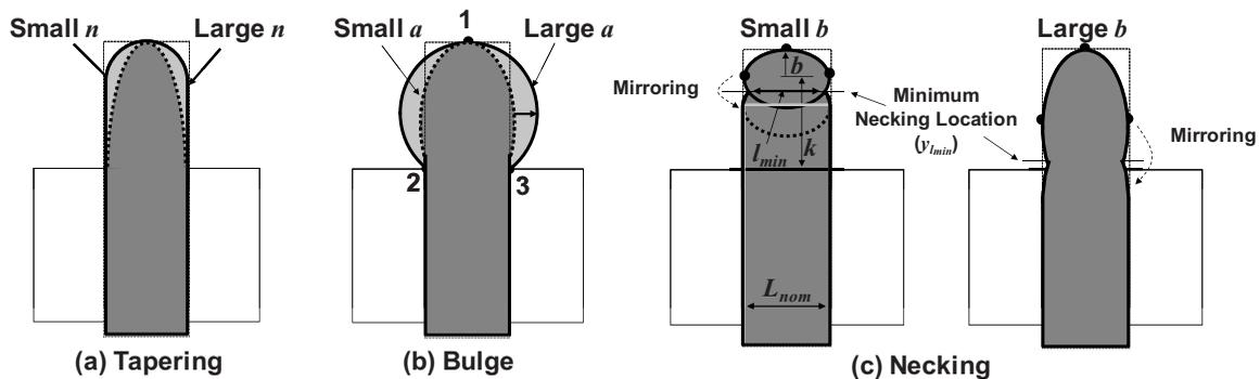
Fig. 5 Line-end shapes represented by the super-ellipse equation.
