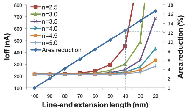
**Fig. 9** Area-leakage trade-off for an SRAM bitcell.
