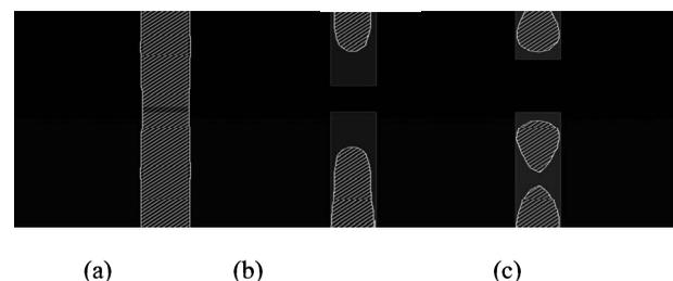
**Fig. 18** Lithographic errors at the line-end. (a) Bridging, (b) line-end shortening, and (c) broken.
