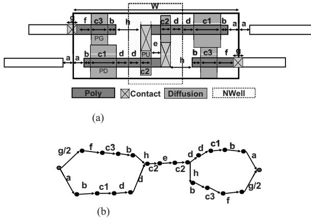
**Fig. 8** SRAM layout and width constraint graph. (a) 6-T SRAM bitcell layout. (b) Width-constraint graph.
