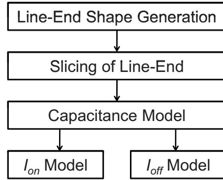
Fig. 2 Line-end extension modeling flow.  $I_{on}$  and  $I_{off}$  can be modeled as functions of line-end extension capacitance.
