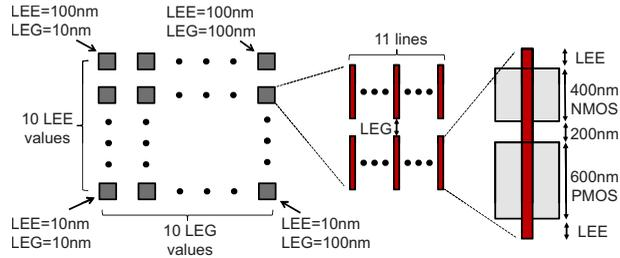
Fig. 13 Layout of the test patterns for OPC/litho simulation.
