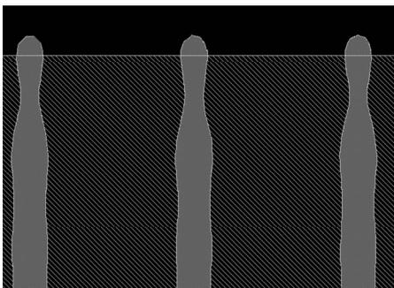
Fig. 19 Significant tapering when the number of fragmentations is 4 and LEG is 20 nm.
