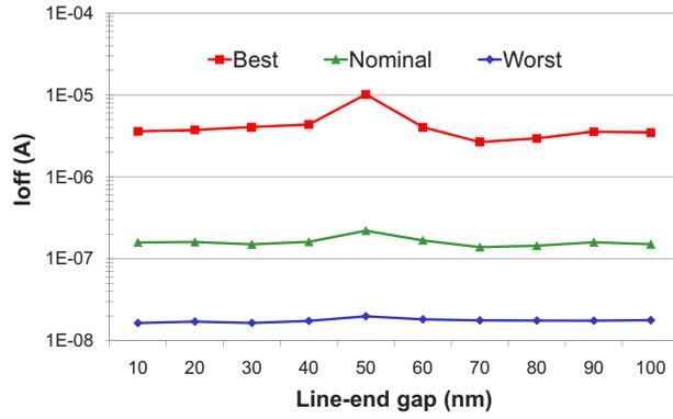
**Fig. 15**  $I_{off}$  variations at best/nominal/worst-case process corners with respect to LEG design rules.
