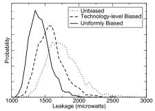
Figure 9. Leakage distributions for unbiased, uniformbiased and technology-level selectively-biased alu128. Note the "left-shift" of the distribution with the introduction of biasing.
