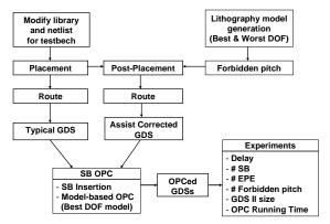
**Figure 5.** The modified design and evaluation flows: Note the added steps of forbidden pitch extraction and post-placement optimization to ASIC design flow
