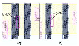
Figure 1. The signed edge placement error (EPE).
