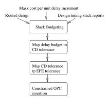
Figure 3. Design-aware OPC flow to find quantified edge placement error tolerances for layout features and drive OPC with them.
