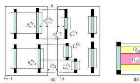
Figure 6. (a) multiple interactions of gate-to-gate, gate-to-field, and field-to-gate, and (b) overlapped area in the region A of (a).
