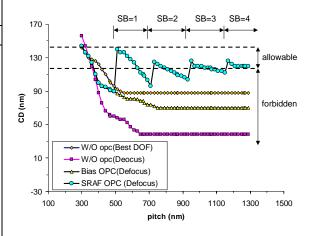
**Figure 8.** Evaluation of proximity plots in through-pitch: Best focus without OPC, worst defocus without OPC, worst defocus with BIAS OPC, worst defocus with SRAF OPC.
