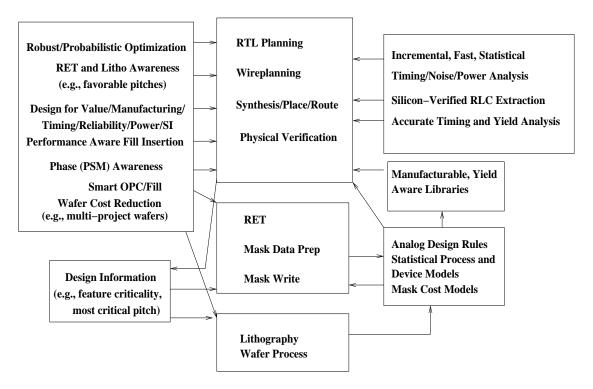
Figure 2: Near-Term Design-to-Manufacturing Flow
