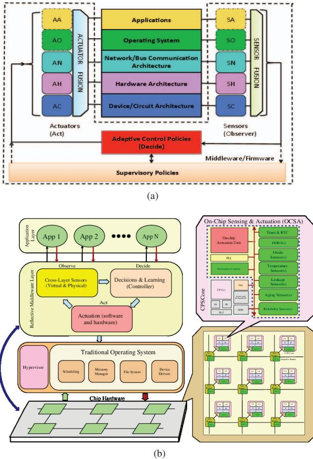
Figure 1: (a)Cross-layer virtual sensing and actuation at different layers of CPSoC (b) CPSoC architecture with adaptive Core, NoC, and the ODA Loop and Middleware.
