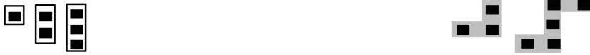
(a) Examples of DSA groups allowed in both 193i and EUV. (b) Examples of DSA groups allowed in EUV but not in 193i.
