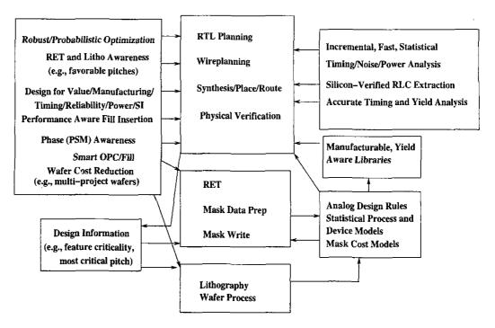
Figure 2: Near-Term Design-to-Manufacturing Flow
