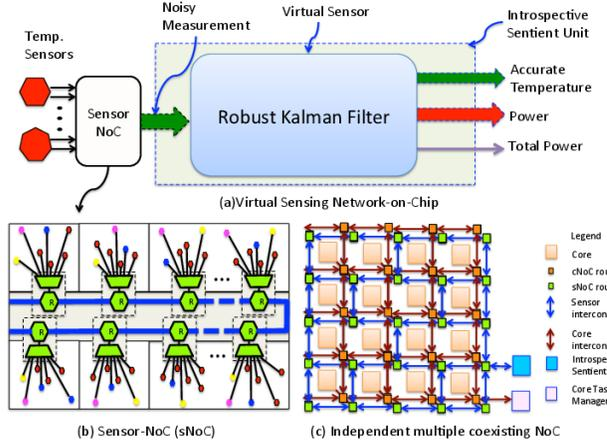
Figure 3. (a)Virtual Sensor Network-on-Chip Architecture (b) Sensor NoC (sNoC) (c) Independent multiple coexisting NoCs in CPSoC.
