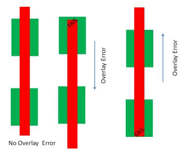
Figure 5. Example of overlay instance scenarios for which failure can occur because of overlay error in both direction
