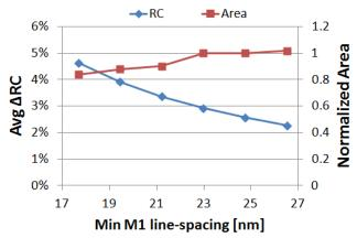
Figure 13. Plot for the average  $\Delta RC$  and the normalized design area for different values of the minimum line-spacing rule.
