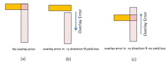
Figure 6. Example of an overlay instance causing failure only in one direction (a) stitch in a L-shaped wire segment (b) for no failure, overlay error should be less than mask overlap length in the given direction (c)no failure in this direction for any value of overlay error
