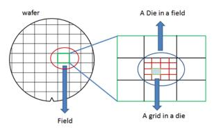
Figure 7. Pictorial representation of wafer, exposure fields, dies and the grid structure on each die.
