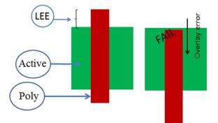
Figure 3. Poly line-end extension rule and failure criteria. The assumed process is one that does not define poly line-ends with a separate cut-exposure.
