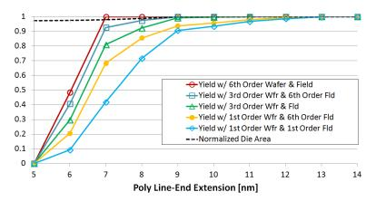
Figure 10. Plots showing the interaction between the polysilicon line-end extension rule and overlay control and their impact on yield and die area.
