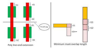
Figure 4. Example of various overlay instances scenarios for poly line-end extension and minimum mask overlap length
