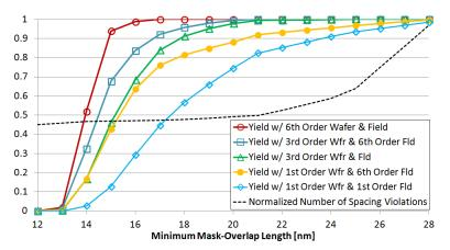
Figure 12. Plots showing the interaction between the overlap-length rule and overlay control and their impact on yield and DP-compatibility of the design at the nominal line-width of 23nm.
