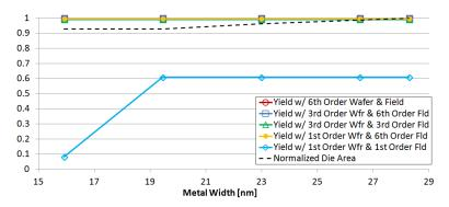
Figure 11. Plots showing the interaction between the minimum line-width rule and overlay control and their impact on yield and layout area of the design with minimum overlap-length rule of 14nm.
