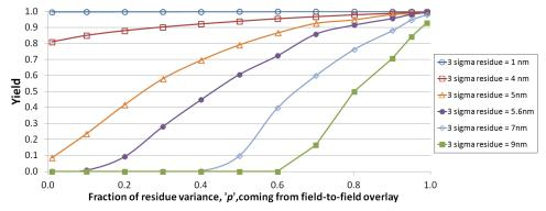
Figure 9. Plots showing the effects of the breakdown of overlay among field-to-field and within-field overlay components for different overlay-residue values.
