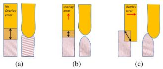
Figure 2. Example of a stitch (drawn and on-wafer) in a vertical line (a), a possible failure with overlay error in Y direction that may occur after line-end pullback (b), and a possible failure with overlay error in X direction due to narrowing (c).
