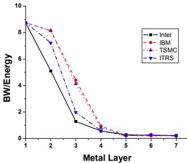
Figure 14: BW/Energy in 90nm technology
