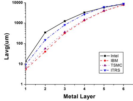
Figure 3: Average wire length in 130nm technology
