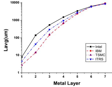
Figure 4: Average wire length in 90nm technology
