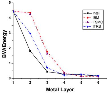
Figure 13: BW/Energy in 130nm technology
