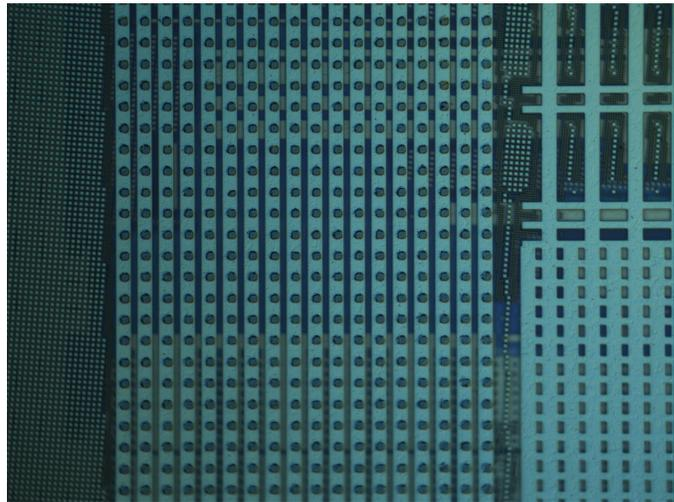
**Fig. 7: Micrograph of sheared-off dielet shows excellent alignment accuracy during bonding.**
