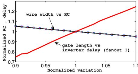
Figure 2. Sensitivities of wire RC and gate delay to patterning variation.
