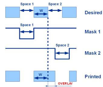
Figure 11. Example showing translation of overlay error into line-width variation in negative DPL process.
