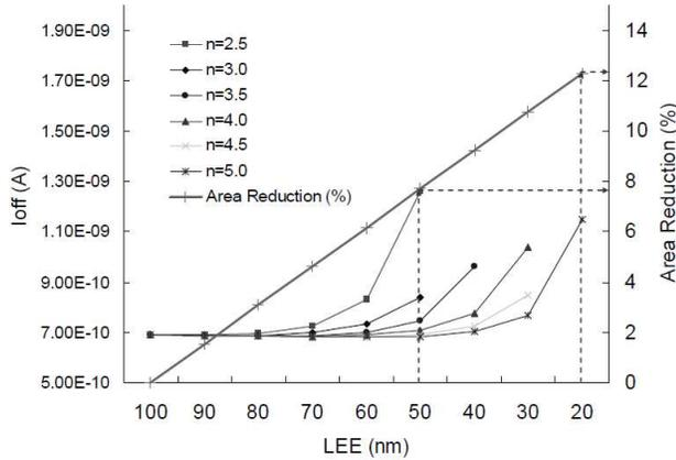
Figure 8. Area-leakage tradeoff for a 6T SRAM bitcell. Higher N implies better OPC and more rectangular line-ends.
