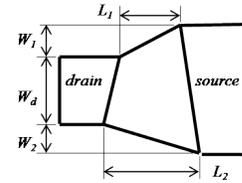
Figure 6. Description of a transistor with combined active and poly rounding.
