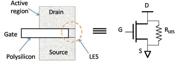
Figure 9. A transistor suffering LES and its equivalent circuit.
