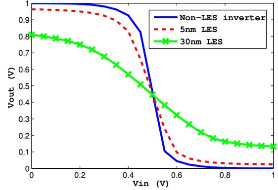
Figure 10. Voltage transfer curves for 45nm LES and nominal inverters.
