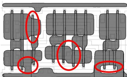
Figure 1. Lithography simulation contour showing non-rectangular gate transistors and line-end imperfections in a layout at 90 nm technology node. [60].
