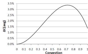
Figure 13. Average coupling capacitance variation in positive DPL process as a function of routing congestion.
