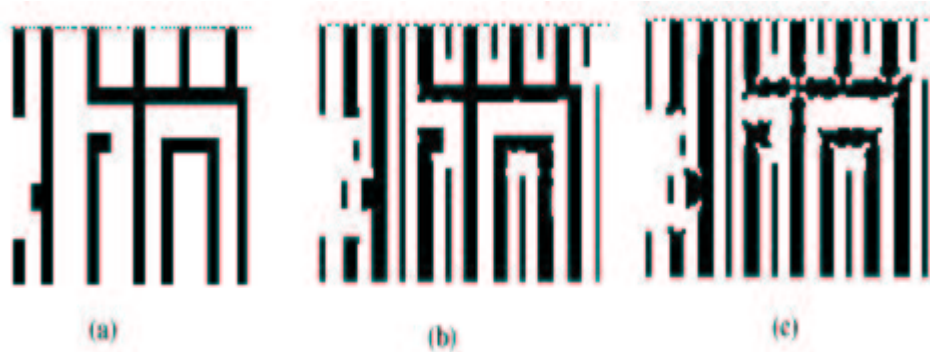
Figure 4: An example of three levels of OPC. 19 (a) No OPC, (b) Medium OPC, (c) Aggressive OPC.
