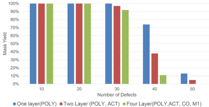
Figure 5. Comparison of mask yield after defect avoidance when multiple layers of a design is patterned using EUV lithography.
