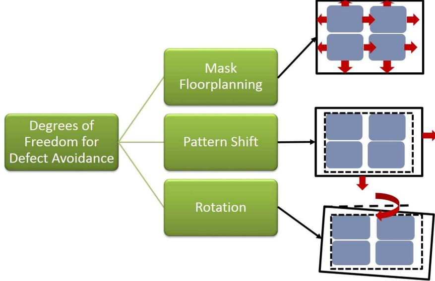
Figure 1. Summary of three degrees of freedom for avoiding EUV mask defects.
