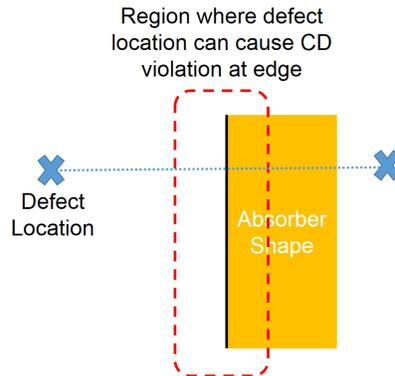
Figure 2. Illustration of non-convexity of CD constraint showing that two feasible defect locations and the segment connecting them crosses through the prohibited region for an absorber edge.
