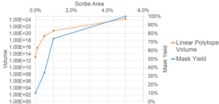
Figure 8. Volume of Linear Polytope and Mask Yield for 40 defect mask with respect to Maximum Allowed Scribe Area.
