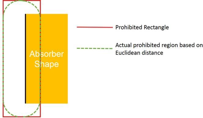
Figure 4. Pessimism of prohibited rectangle construction compared to true prohibited region based on Euclidean distance for one absorber edge.
