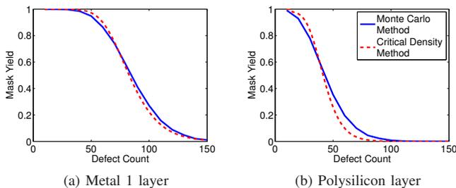
Fig. 4. Mask yield versus defect density for two layers of  $s1423$  design
