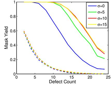
Fig. 2. Comparison of pre-pattern shift (dashed lines) and post-pattern shift (solid lines) mask yield of four parallel line layouts with same prohibited region density but different  $\sigma$  of Gaussian width.
