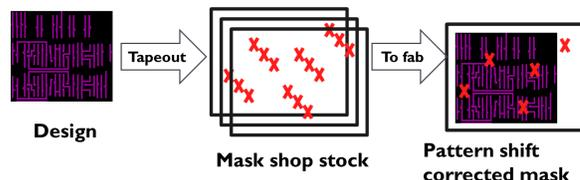
Fig. 1. Set of steps involved in a EUV mask shop involving pattern shift based mask defect mitigation.
