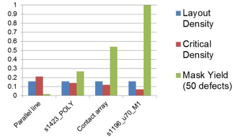
Fig. 5. Illustration of impact of regularity on critical density (and consequently, mask yield) for layouts with same density.
