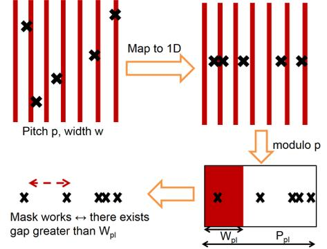
Fig. 3. Mapping mask yield estimation of parallel line to maximal spacing distribution.
