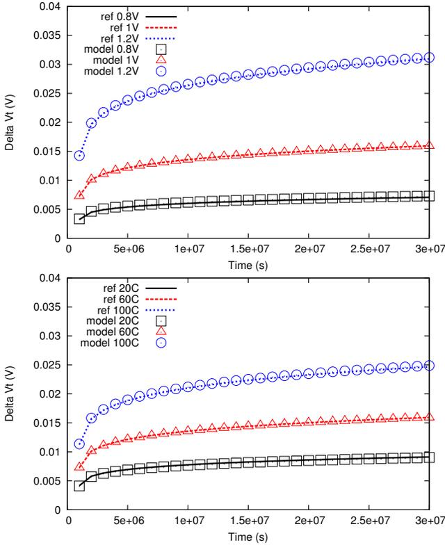
**Figure 3: Threshold voltage degradation obtained from reference design manual vs. fitted model in (1) under different supply voltages at 60°C (top) and temperatures at 1V (bottom)**
