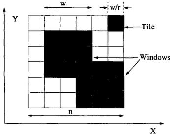
**Figure 1:** In the fixed  $r$ -dissection framework, the  $n$ -by- $n$  layout is partitioned by  $r^2$  (here,  $r = 3$ ) distinct overlapping dissections with window size  $w \times w$ . This induces  $\frac{nr}{w} \times \frac{nr}{w}$  tiles. Each dark-bordered  $w \times w$  window consists of  $r^2$  tiles.
