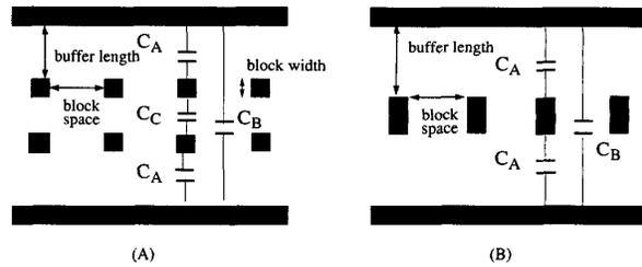
**Figure 2:** Example configurations of floating dummy fill.
