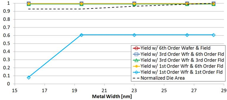
Figure 11. Plots showing the interaction between the minimum line-width rule and overlay control and their impact on yield and layout area of the design with minimum overlap-length rule of 14nm.
