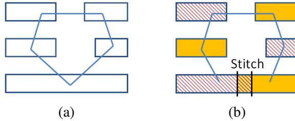
Figure 1. Example of a DP-problematic layout pattern with an odd cycle in its conflict graph (a) that was broken by introducing a stitch (b).
