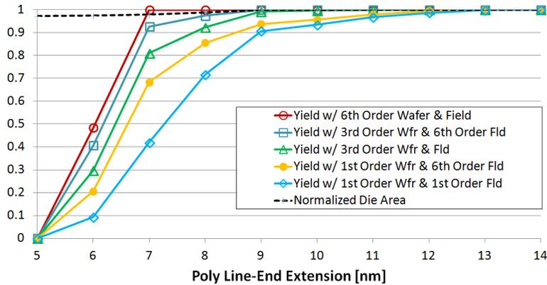
Figure 10. Plots showing the interaction between the polysilicon line-end extension rule and overlay control and their impact on yield and die area.
