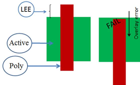
Figure 3. Poly line-end extension rule and failure criteria. The assumed process is one that does not define poly line-ends with a separate cut-exposure.
