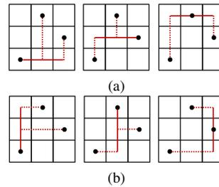
Figure 2. Example of possible wiring solutions with single-trunk Steiner-tree topology for a three-pin net using (a) horizontal trunks and (b) vertical trunks.
