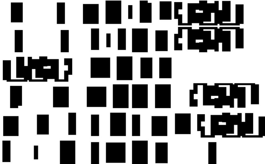
Figure 8: Trim-mask layout snippet where simple large blocks correspond to cells with unidirectional poly and more complex shapes correspond to flip-flops with bidirectional poly-routing.
