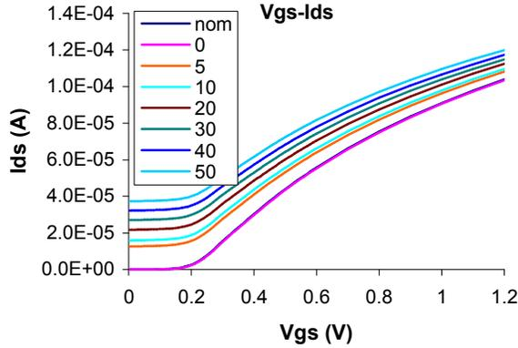
Figure 3. Id-Vgs characteristics of LES devices (NMOS).
