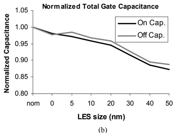
Figure 2. Ion/Ioff current in NMOS and PMOS devices (a) and normalized gate capacitance (b) with LES.
