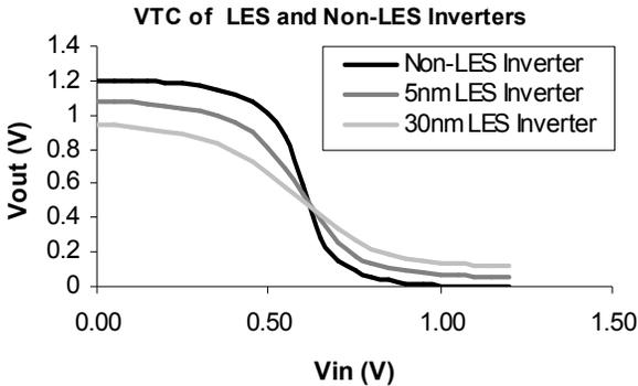
Figure 5. Voltage transfer characteristics of LES and non-LES inverters.
