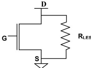
Figure 4. Equivalent circuit model for the LES device.
