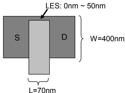
Figure 1. Device structure for TCAD simulations.
