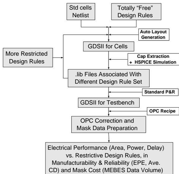
Figure 1: ASIC design flow targeting RDR evaluation.
