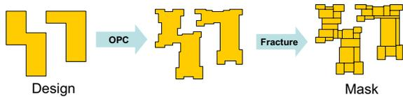
Figure 5: Mask data preparation (post OPC).
